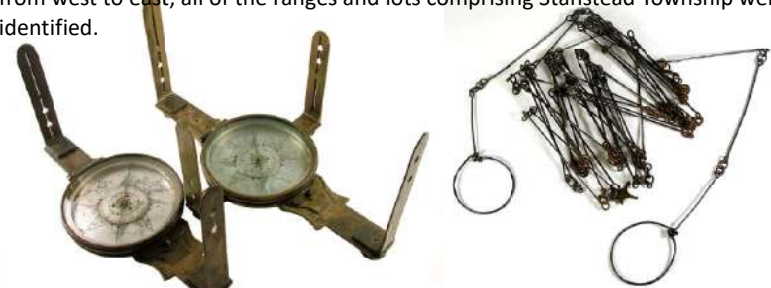
Essential survey equipment of the era. At left are surveyor's magnetic compasses (or interferometers). At right a Gunter's Chain, used to measure distance. A full chain was 66 feet long, and was divided into 100 links. One statute mile was equal to 80 chain lengths. The chain had to be pulled taught, so the chainmen had to have strong arms.
